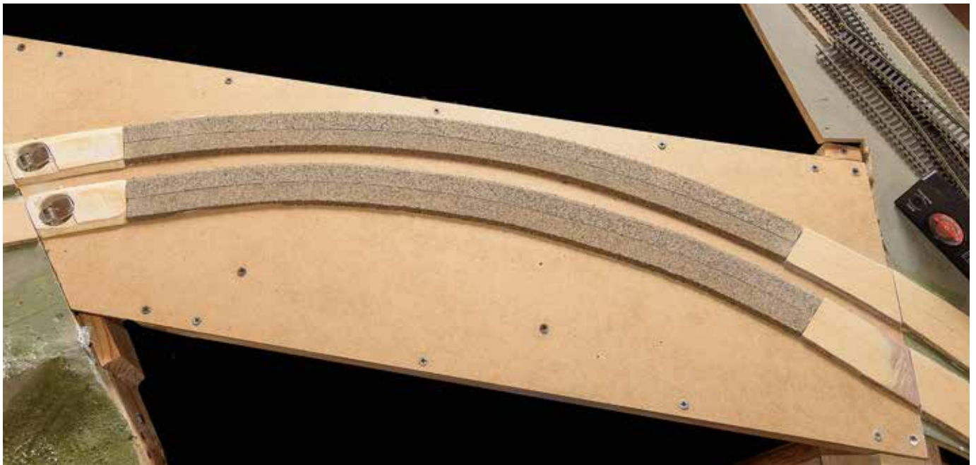
6 A versatile solution. The tracks can be curved or straight relative to the joint on the lift-up section. Two Euro-style hinges were used on this lift-up section. The cup section of the hinges is visible at left.
