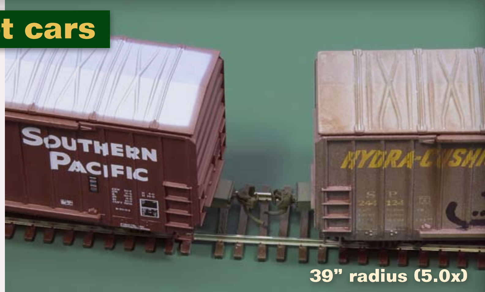
FIGURE 18: For all practical purposes, coupler alignment on the 5.0x curve for the 50 ft boxcars matches that of straight track.
