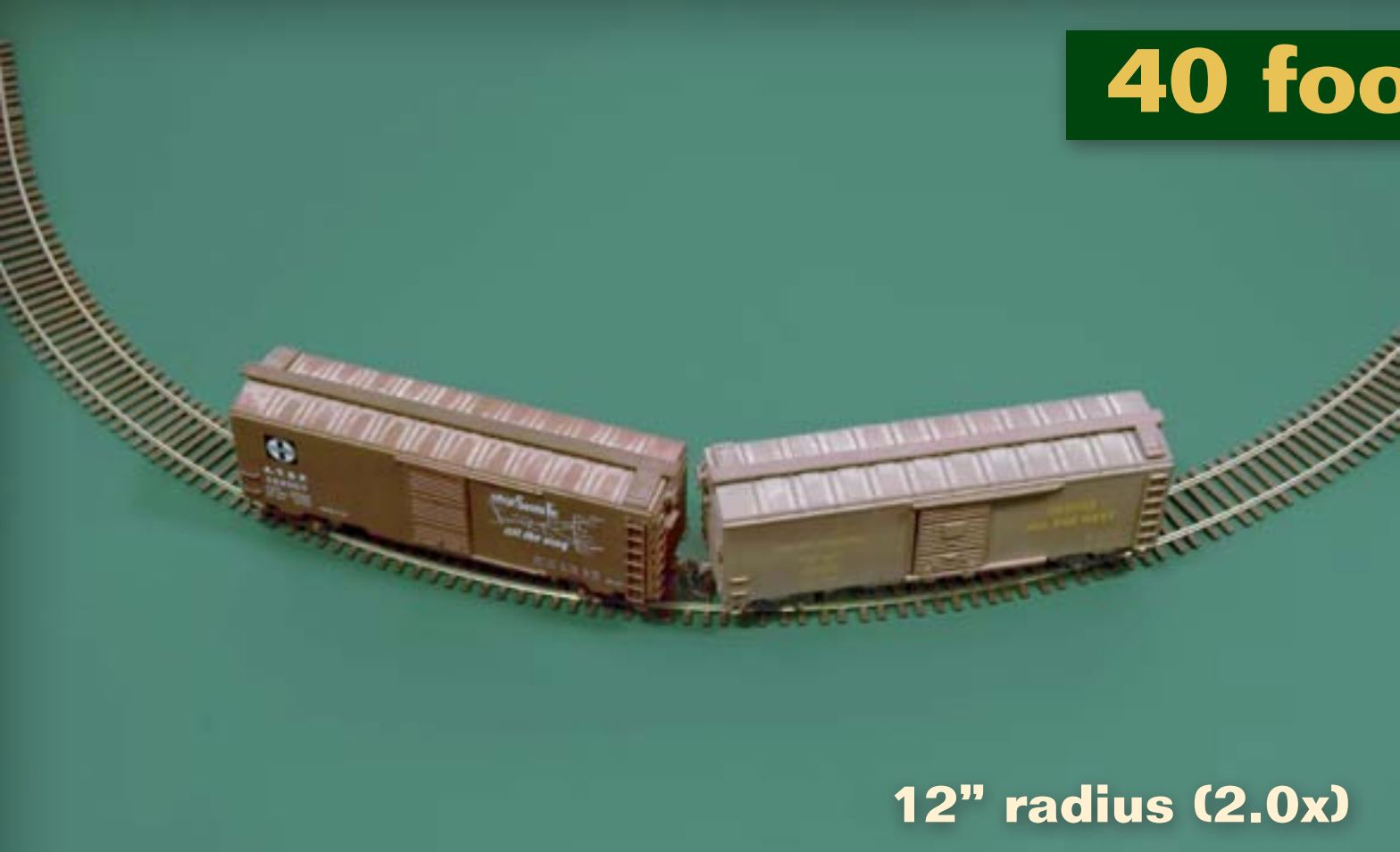
FIGURE 5: Getting the cars on the track takes some care, and the flanges rub against the railheads with noticeable friction.
