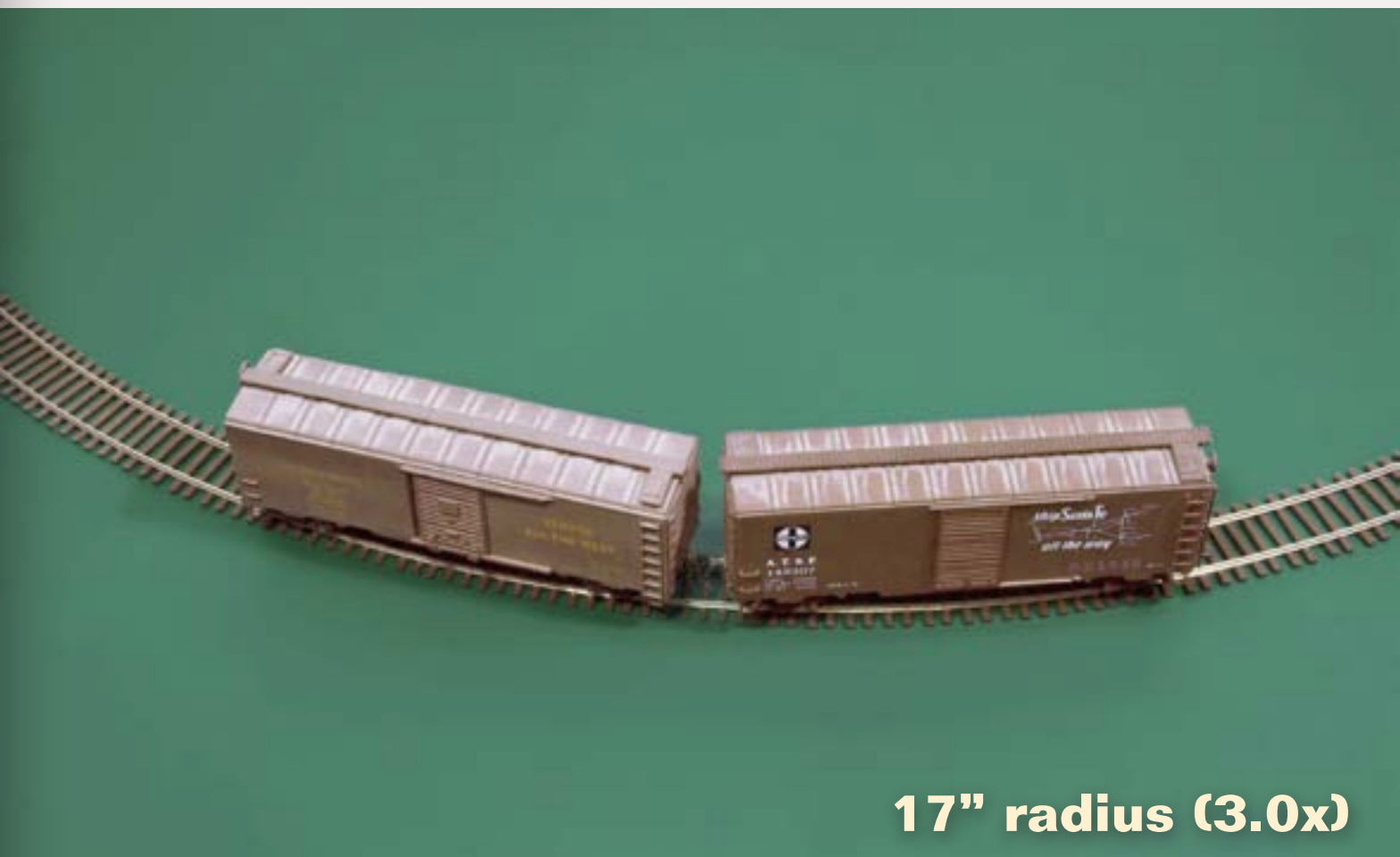
FIGURE 7: The cars roll freely at the 3.0x radius of 17". The cars couple with a bit of coaxing to make sure the couplers are aligned.
