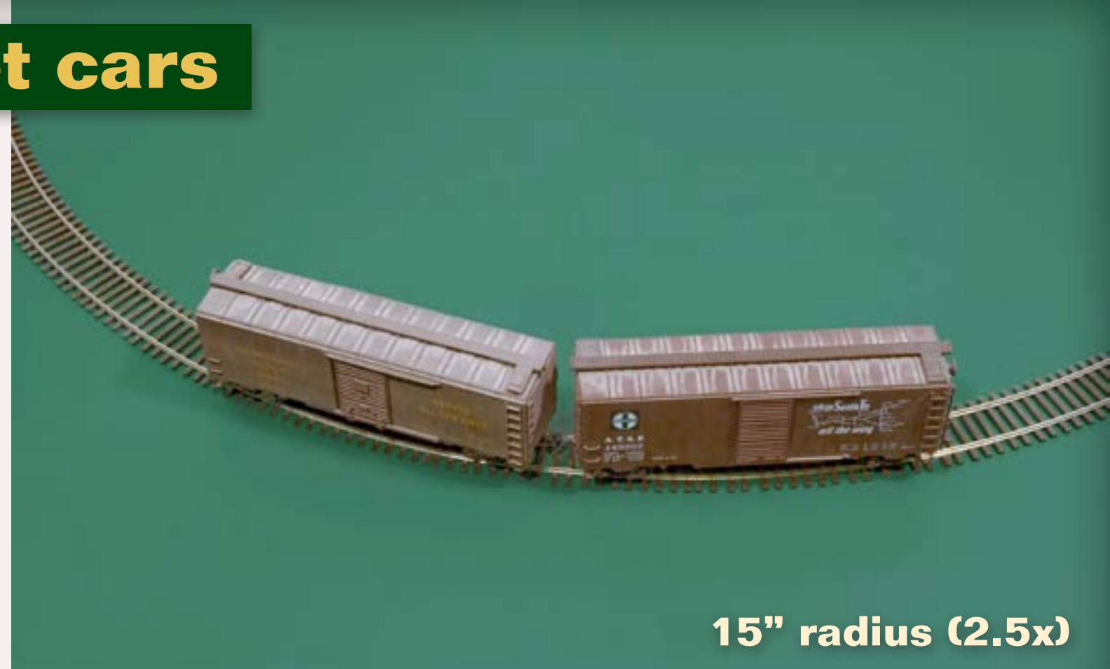
FIGURE 6: The cars track without friction at this radius, proving the 2.5x radius guideline works well in predicting car tracking behavior.
