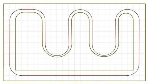
By contrast, below is a second diagram showing the footprint where only ONE serpentine peninsula was used. Note the much longer linear runs that we so desperately need.
