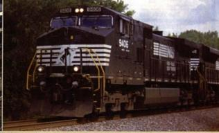
By 1963, many of the New York Central's switchers had a rotary beacon on the front edge of the cab roof to make them more visible at night. This Norfolk Southern Dash 9-40CW displays the current three-light system with a headlight and two alternately flashing lower lights to capture motorists' attention. Jim Hediger photos
