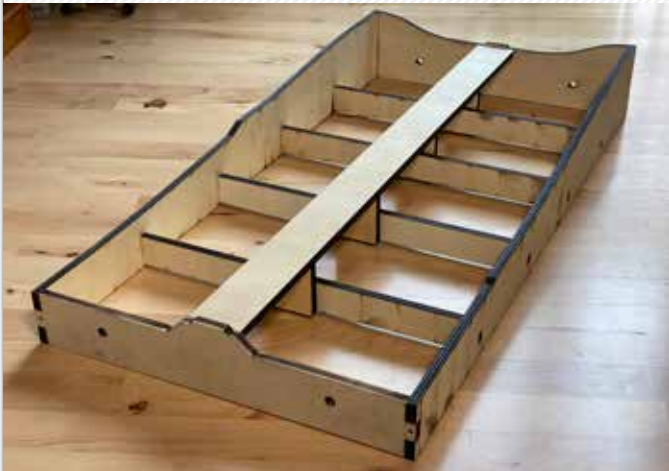
After Pelle made drawings for the module frame parts, he had them laser-cut. The framing is 1/2" birch plywood.
