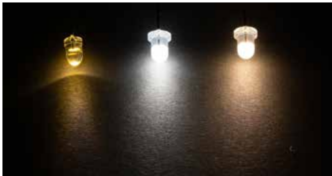
1 Left to right: NCE (ncedcc.com) WWLEDx20 Warm White, SoundTraxx (soundtraxx.com) No. 810133 Sunny White, and SoundTraxx No. 810134 Golden White. Allan Gartner put a 1,000 ohm resistor in series with each of the LEDs shown here. You can change the resistor value to control the LED's brightness. The LED from NCE is more "point source" than the "diffuse" LEDs from Soundtraxx.
