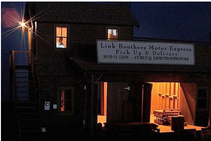
Warehouse lighting looks just right using 12 volt incandescent lamps.
