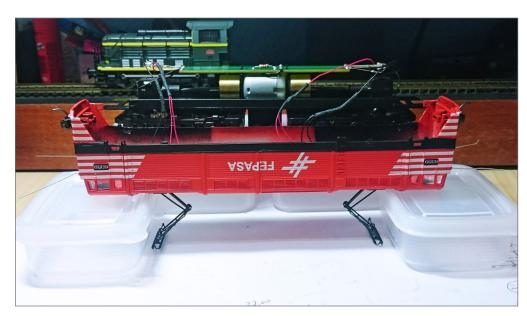
5. Start by disassembling the locomotive or rail car according to the manufacturer's instructions.
