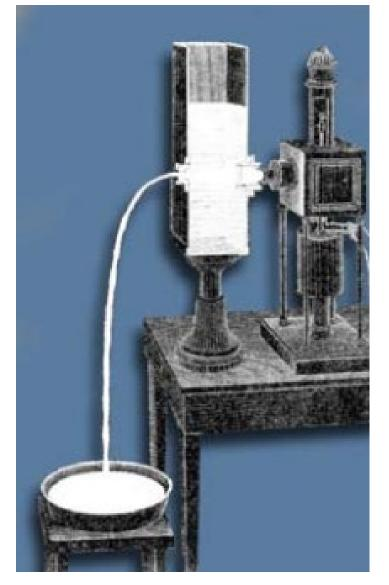
3. In 1870, the English physicist John Tyndall demonstrated the principle of guiding of light by means of a simple experiment. Using a leaky container with water, a bucket and a light source, Tyndall observed that the beam was illuminated through the hole in the container.
