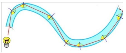
4. The optical fiber is glass or plastic polymer. Optical fibers have a transparent core surrounded by cladding with a lower refraction index. Light is contained in the core by the phenomenon of total internal reflection.
