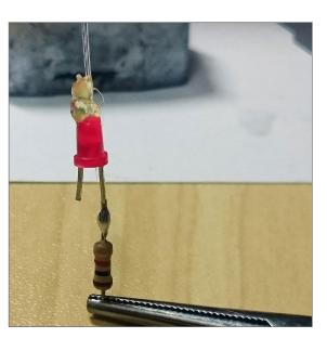
7. We will install two 2.8mm red LEDs, one in each cabin, to serve as the light sources. Solder a resistor to the positive pole of each LED to limit the inflow voltage. Cut two 100mm (about four inches) pieces of optical fiber and attach them to the LED housings with a drop of hot glue or superglue. Keep the soldering iron away from optical
