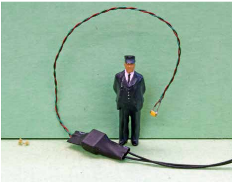
John posed an HO scale conductor figure next to the LED and resistor he used for his fusee project. The LED is roughly the same size as the figure's hat.
