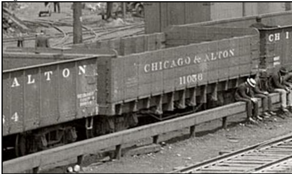
The 1,100 cars of the 11000-series were the general workhorse gondolas of the C&A until the 1920s. When built the Alton was also buying all-steel gondolas for the mill trade. These all-wood, flat-bottomed cars were built to a fairly common industry design, and would survive without extensive rebuilding until 1930.
