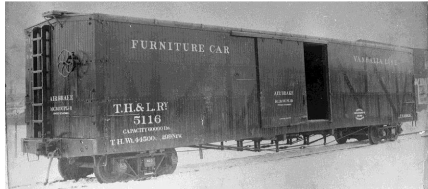
TH&L 5116 was one of 20 cars built by ACF's Terre Haute IN plant in December 1899. Only 5,500 boxcars over 45 feet long were in service by 1900. (ACF builder's photo, Al Westerfield collection)
