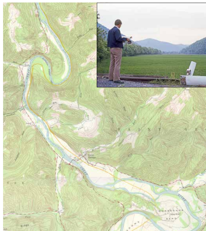
The U.S. Geological Survey 15-minute quadrangle map for St. George, W.Va., shows the abandoned Rowlesburg & Southern right-of-way along the east bank of the Cheat River as a broken line or dirt road and the open area where the AM's main classification and coal-marshaling yards were located. Tony's field trip to that location (inset) confirmed the map's information.
