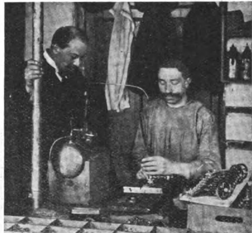
TESTING MODEL STEAM ENGINES BY STEAM FROM A SEPARATE BOILER.
