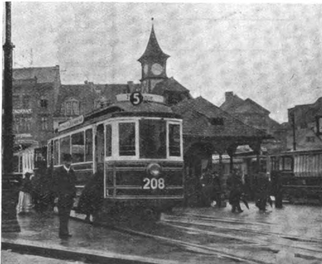
ELECTRIC TRAM-CARS AT NUREMBERG, SHOWING A TYPICAL TRAMWAY STATION WITH WAITING-ROOM, A SUMMER TRAILING-CAR, AND THE GLASS WEATHER-BOARD FOR THE CAR DRIVER.
