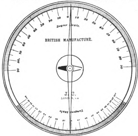
FIG. 6. SHOWING PLAN OF COMPASS-BOX; WITH SCALE, NEEDLE AND POINTER FOR TANGENT GALVANOMETER.
