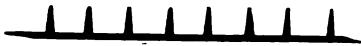
FIG. 22.—THE "SERVE" FLUE TUBE DURING MANUFACTURE, BEFORE IT IS ROLLED UP AND WELDED.
