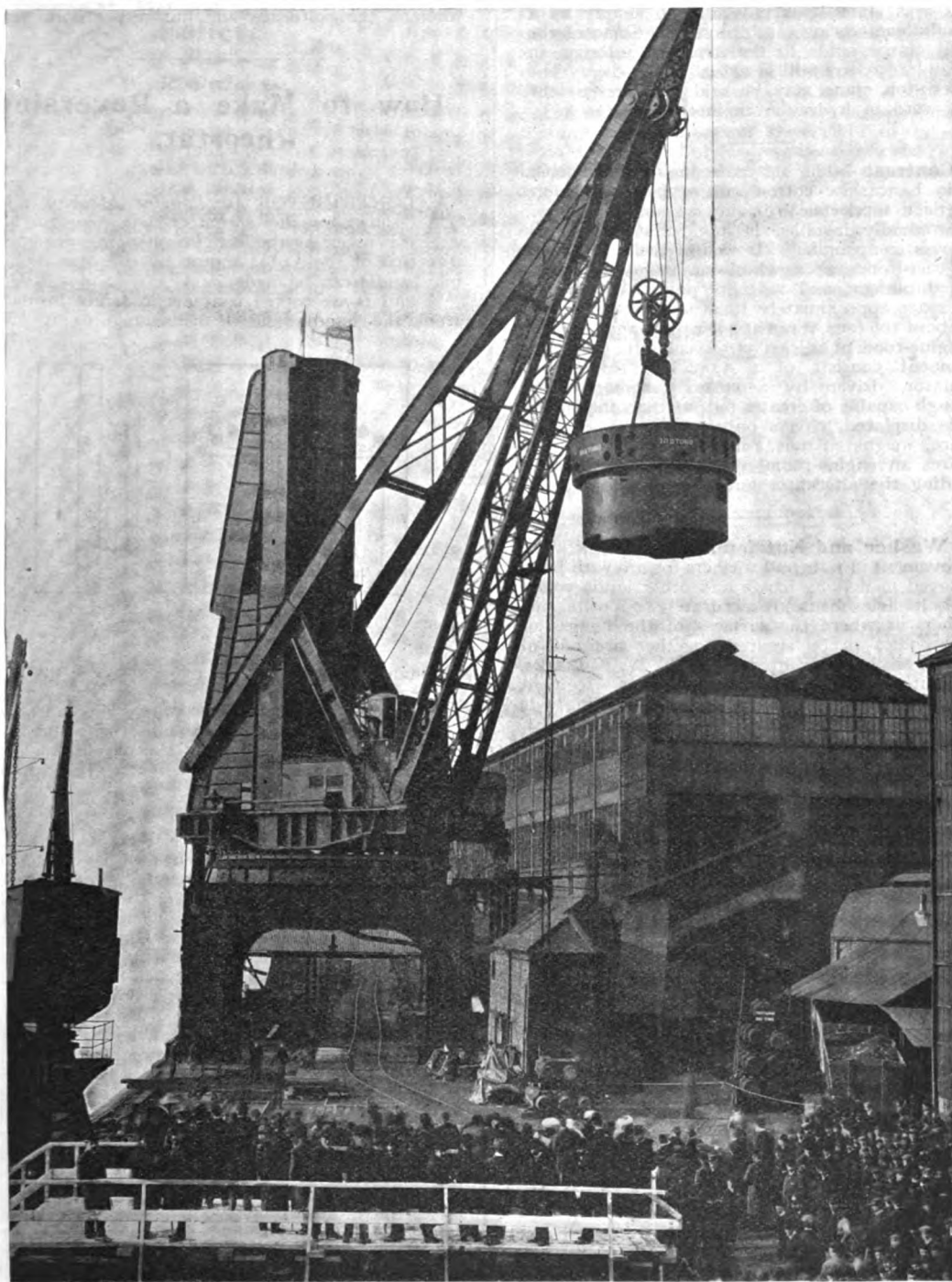
THE NEW 150-TON HYDRAULIC CRANE. (Built by Sir W. G. Armstrong, Whitworth & Co., Ltd.)
