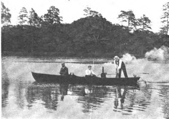
SHOWING ROWING BOAT, FITTED WITH A BOILER AND ENGINE.
