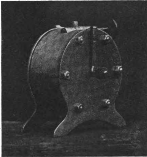
FIG. 2.—VIEW SHOWING EXTERIOR OF MODEL WATER TURBINE. (See page 65.)
