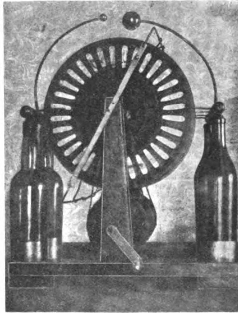
TWO VIEWS OF SIX-PLATE WIMSHURST MACHINE.
