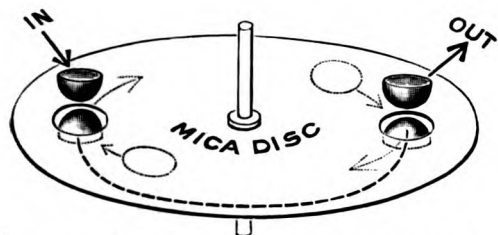
FIG. 3.—MICA DISC OF MR. LESLIE MILLER'S VALVE.
