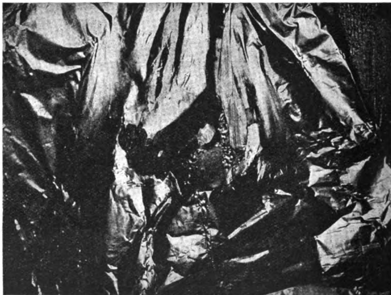
FIG. 56.—TINFOIL SHEET AFTER BEING MELTED BY INDUCED EDDY-CURRENTS. (About half actual size.)
