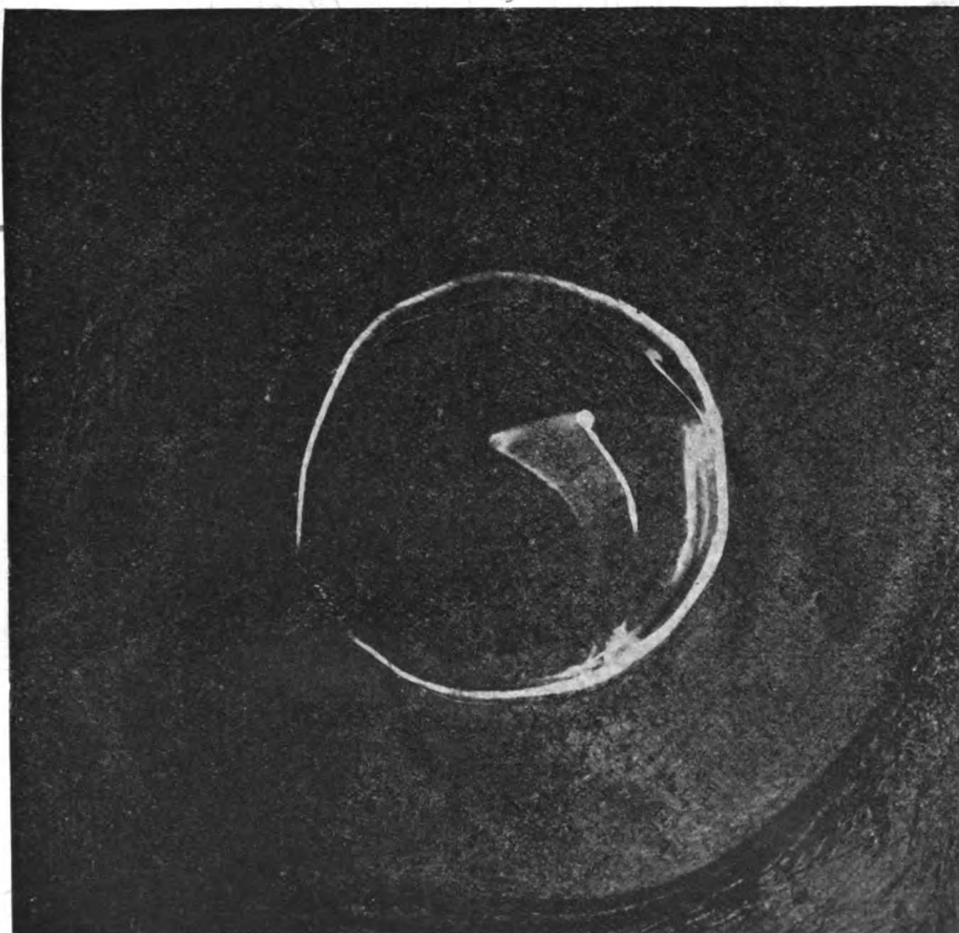
FIG. 57.—IRON RING FUSED BY EDDY-CURRENTS. (About half actual size.)
