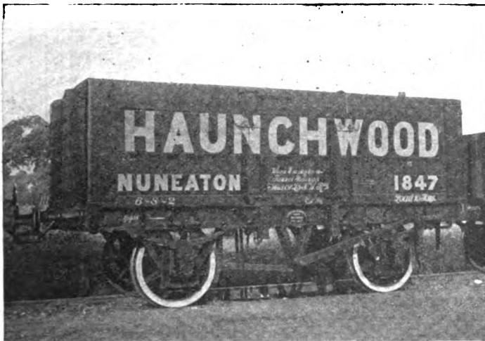
FIG. 8.—HIGH-SIDED 10-TON PRIVATE WAGON, WITH TOP FLAP OVER DOOR.
