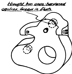
FIG. 7.—CAST-IRON CENTRES USED WHEN TURNING THE BIG-END JOURNALS.
