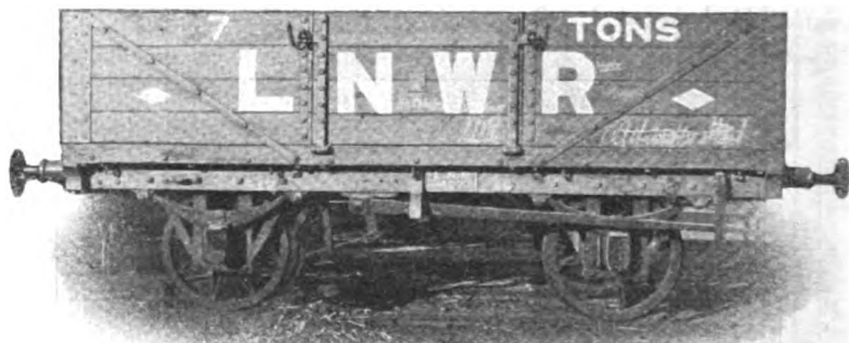
FIG. 23.—A PHOTOGRAPH OF L. & N.W.R. 7-TON OPEN GOODS WAGON.
