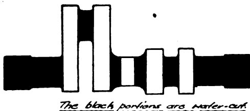
FIG. 15.—CRANK-AXLE SHOWING THE PORTIONS WHICH ARE WATER-CUT.
