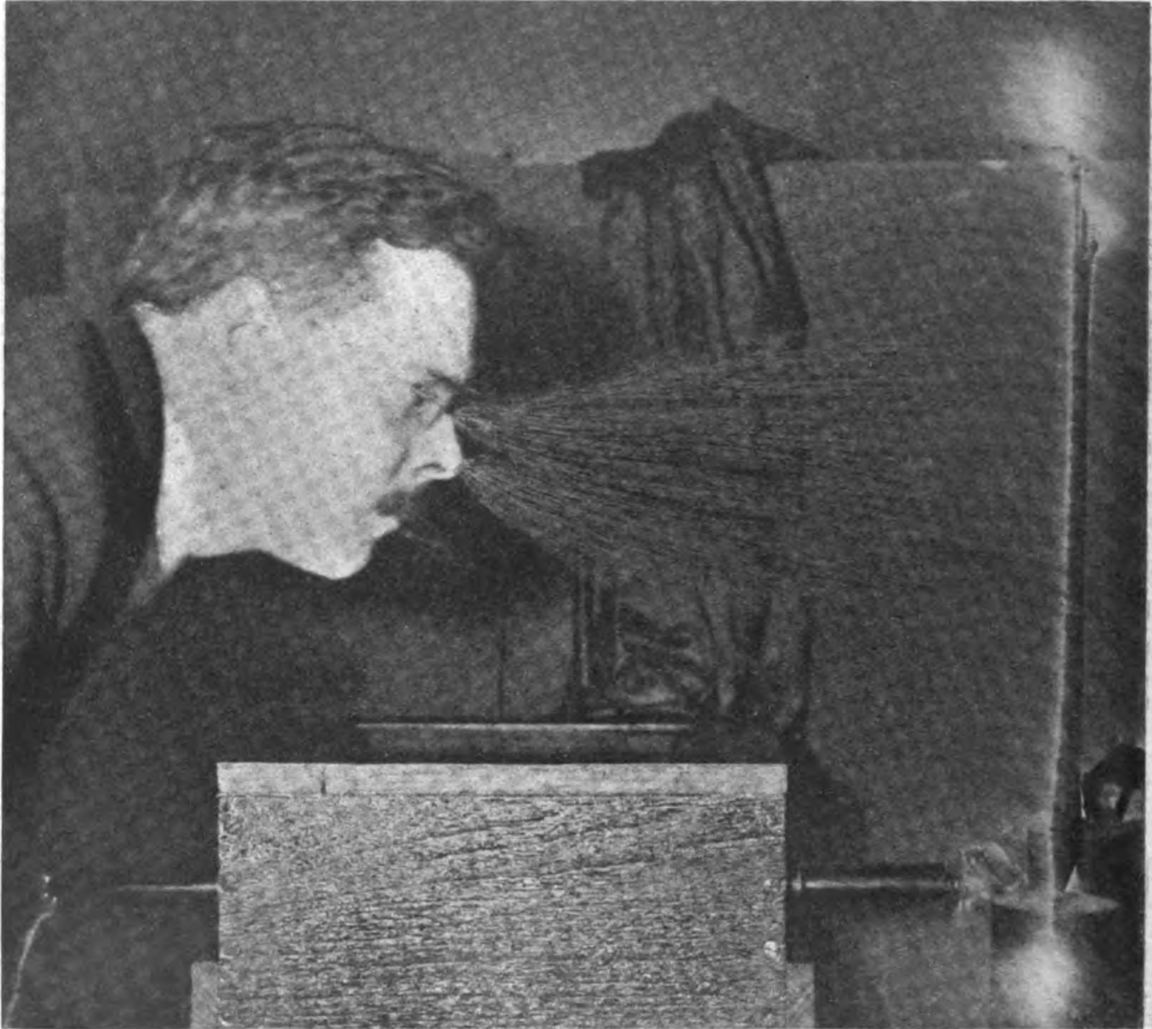
FIG. 70.—TREATED PHOTOGRAPH OF BRUSH DISCHARGES FROM FACE. ( Exposure about 1 second. )
