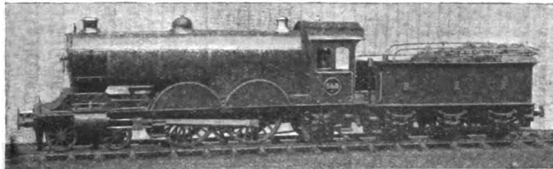
FIG. 4.—MODEL N.E.R. "ATLANTIC" LOCOMOTIVE, No. 649. ( \frac{1}{2} -in. scale, 2\frac{1}{2} -in. gauge.)
