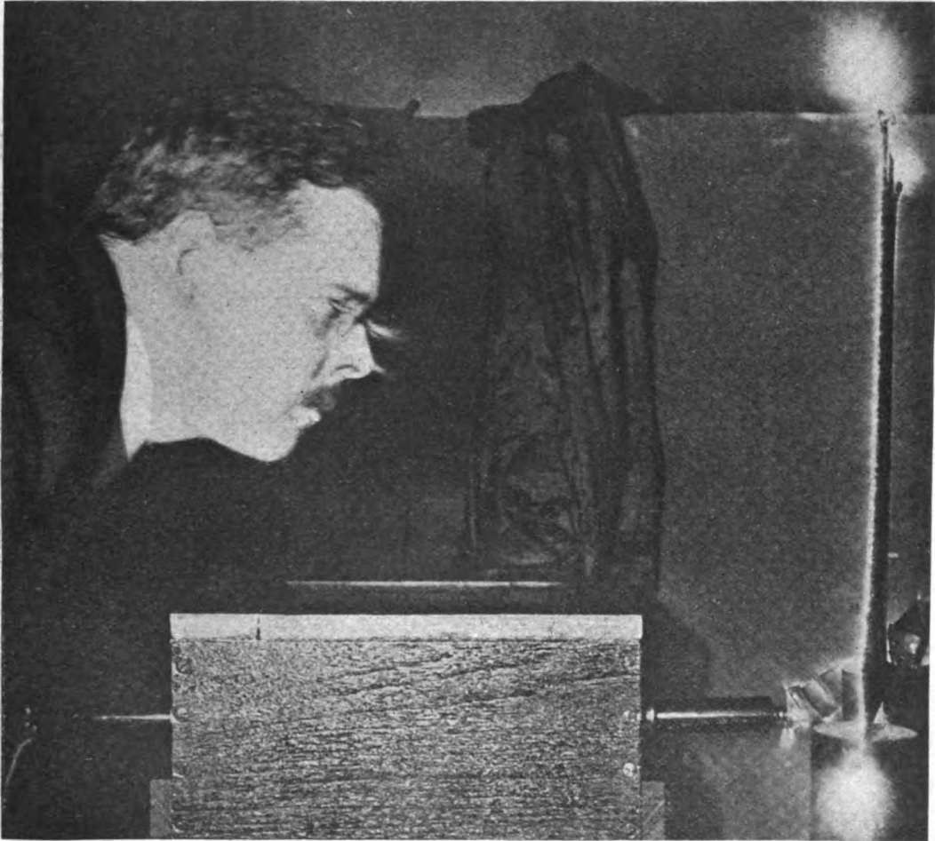
FIG. 69.—UNTOUCHED PHOTOGRAPH OF BRUSH DISCHARGES FROM THE FACE. (Exposure about 1 second.)
