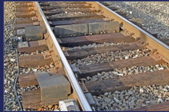
8. The modern radio alarm defect detector uses a group of sensors to measure journal temperatures and a series of upright paddles to detect dragging equipment.
