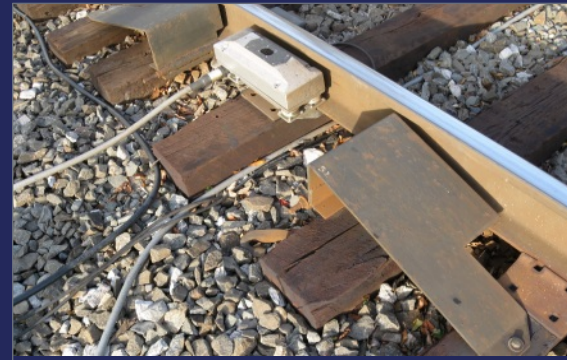
7. Closeup of an axle heat sensor.
