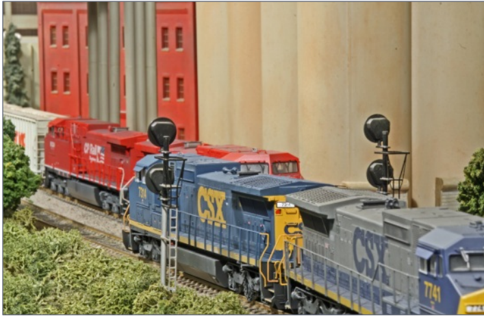
14. CSX Q300 passes the waiting CP train as it enters the controlled siding at Oak Tree. Sidings on a single-track railroad allow trains to pass each other and
