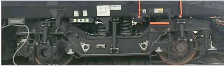
18. EMD first used this modern truck on the F125 commuter locomotives built from 2015 thru 2021 for the Southern California Metrolink. Note the paired coil bolster springs and the use of three automotive style shock absorbers.
