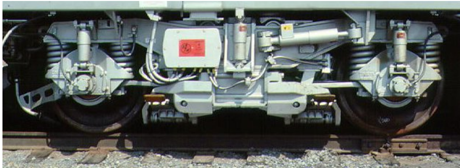
30b. GE-Krupp truck with third-rail shoes for use on GE's P32AC-DM, (AC traction, Dual Mode) built for Northeast Corridor service. The shoes allow the P32AC-DM to switch over to electric only mode as it approaches the tunnels leading to New York's Penn Station.
