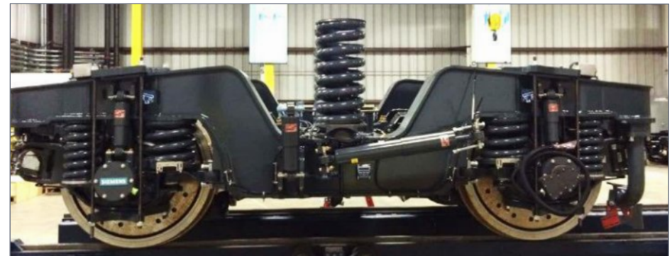
42a. Siemens-Mobility SF4 two-axle two-motor truck.
