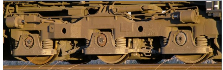
33a. GE's three-motor Hi-Ad (high adhesion) floating-bolster truck was introduced in November 1993 with the release of the microprocessor-controlled third-generation Dash 9-44 units. Subsequent applications include GE's ES44 series launched in 2003 and the ET44 series that followed in 2015. Dofasco worked with GE in developing this truck. In addition to conventional springs, the new truck had a secondary suspension system consisting of four stacks of rubber pads connected directly between the truck and the locomotive under frame.
