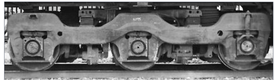
32a. Identified as model FB-3, this floating-bolster truck first appeared in 1956 under GE's U30C. It continued to be used on C-C locomotives through the Dash 8 series. GE used castings made by both Adirondack and Rockwell. Spotting features of the Adirondack FB-3 frame include a boxy shape above the outer axles and two widely spaced non-functional holes in the casting.
