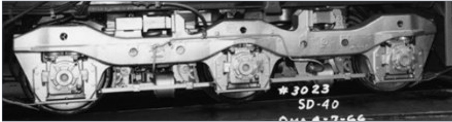
20b. The “teeth” disappeared on latter versions of EMD’s Flexicoil truck as seen on this Union Pacific SD40. Placement of brake cylinders and single-shoe or clasp brakes also altered the appearance of the Flexicoil truck.
