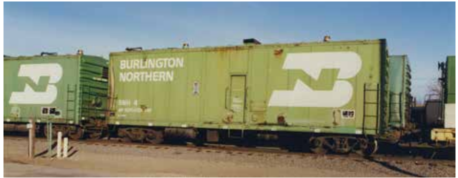
Burlington Northern car BNH 4, seen at Grand Forks, N.D., in 1996, was built in 1955 as Great Northern boxcar no. 5158. It was converted to an air repeater car in 1971. Note the manway door and stirrup step on the side and the twin indicator beacons on the roof. Cody Grivno photo
