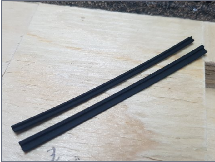
9. Painted 3D-printed "rubber" inserts.
