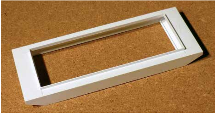
2 James built the coaming, or raised area around the hopper, from .040" x .188" styrene strip. He cemented the strips on edge around the hopper opening using methyl ethyl ketone (MEK).
