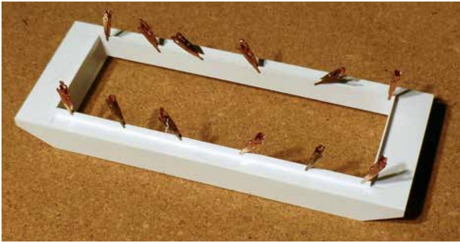
3 Smooth-jaw micro alligator clips held the hopper side in place while the cement cured. James installed the interior ends of the hopper in the same manner.
