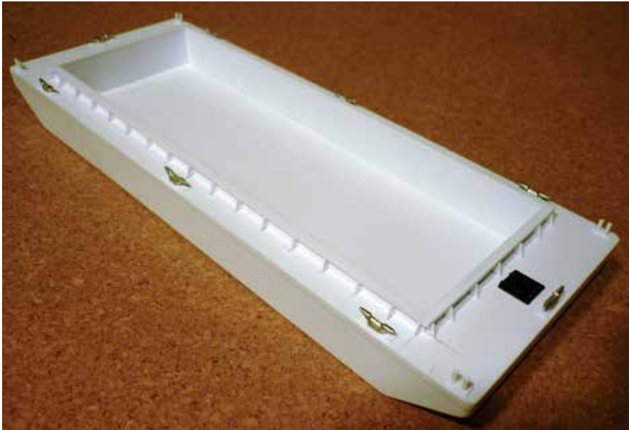
4 A cap along its perimeter and gussets along its sides finish off the coaming, while edging made of HO scale 1 x 10 finishes off the hull. James then added deck details, including an access hatch, cleats, and bollards. The hopper bottom, a rectangle of .030" styrene sheet, has also been installed.
