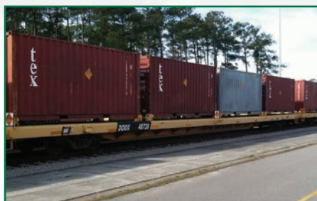
Example of an 89' flat car with four 20' containers on it
