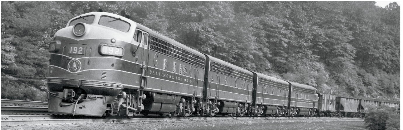
This four-unit set of matched F7s is headed away from us, pushing a Baltimore & Ohio coal train up West Virginia's Cranberry Grade from behind the sturdy steel wagon-top caboose. The flag on the side of the nearest cab unit is a marker indicating the rear of the train. H.W. Pontin photo
