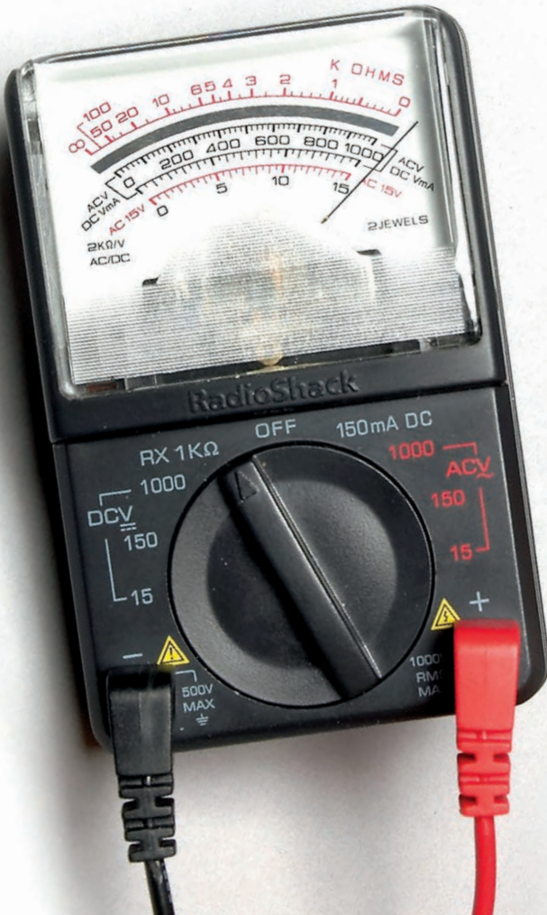
This analog multimeter is set to measure ohms of resistance.
