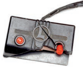
Controller with broken Bakelite case
