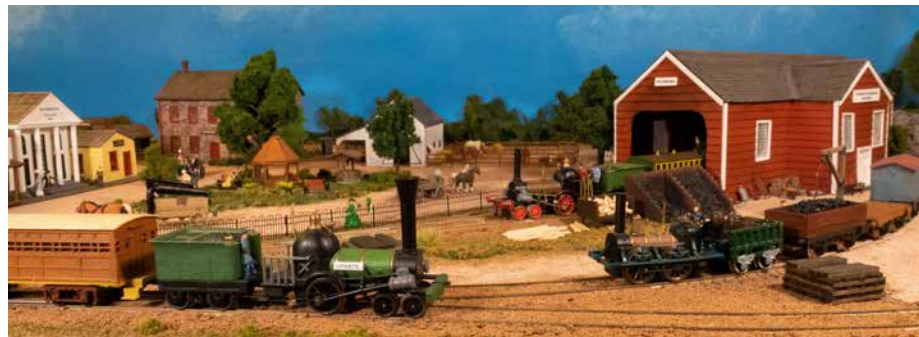
5 An assortment of early first-generation locomotives and rolling stock can be seen outside the Flushing, N.Y., enginehouse. Most rolling stock at the time only had two axles, as seen at right. The passenger car on the left is an early example of bench and aisle seating arrangements.
