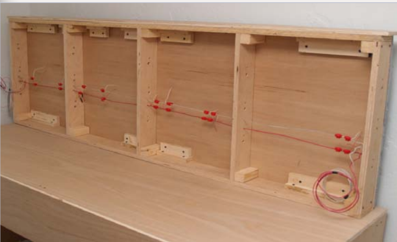
Figure 3. A simple bus under the "mainline" was all that was needed to run both DC and DCC locomotives.
