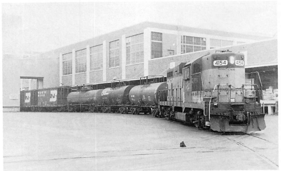
The largest customer on the Chicle Plate Road is Warner-Lambert/American Chicle Group, hence the nickname. On a snowy April day, outbound GP9 4154 spots sugar-laden hoppers in the plant's car shed; the three syrup-carrying tank cars will be spotted elsewhere on the train's return trip.
