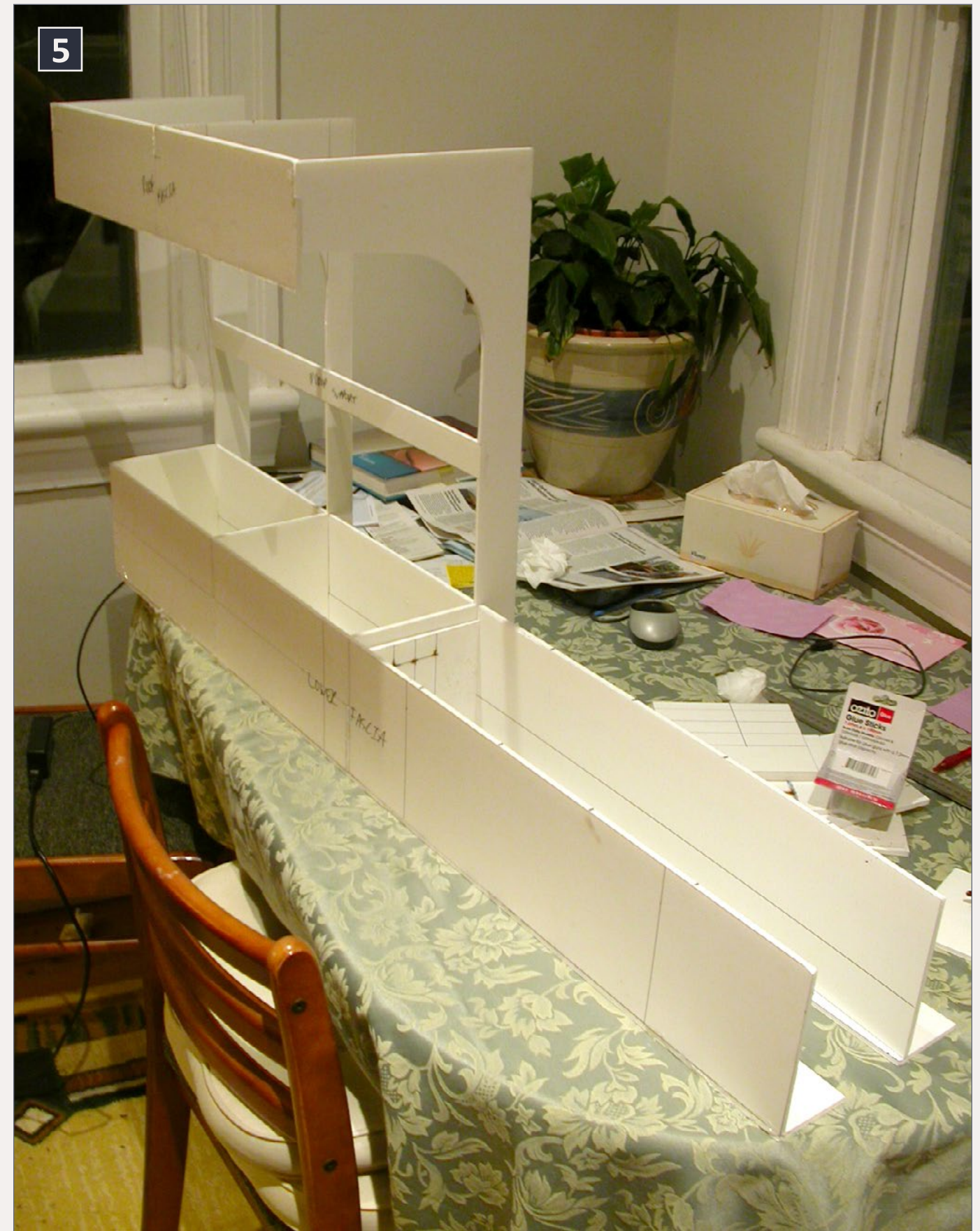
5: Note the overhanging module roof/fascia/lighting pelmet and 6" deep "L-girder" base. Foamcore is imminently suitable for benchwork building as long as basic structural principles are respected.
